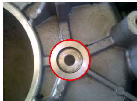
Perbedaan kedudukan idler gear New Flywheel housing dan Old Flywheel Housing
